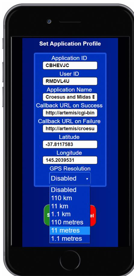
A mobile app, resident on the mobile device also associated with the service, adds the device's current coordinates to a login request page, which it loads into the device's browser. When the user enters his user ID and sends the page, the coordinates are sent to DSS Enterprise.
