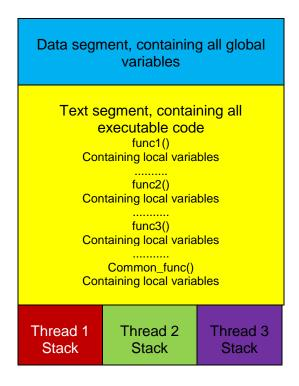
It may be seen that the stack has been split into three independent sections, each of which is allocated to one of the threads of execution. This arrangement, in fact, is the key to the operation of multi-threading, since it provides the means of separating global and local variables.
