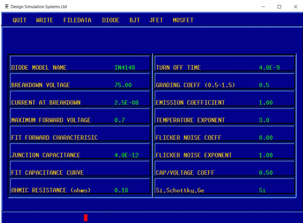
Displays the diode menu. The SPICE parameters are derived from simple calculations, based on the data sheet values entered, and only the capacitance curve is fitted
